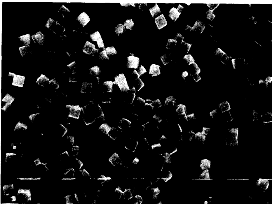
FIG. 1. Scanning-electron micrograph of NaA-1 zeolite. Each scale bar corresponds to 10 \mu\text{m} .
